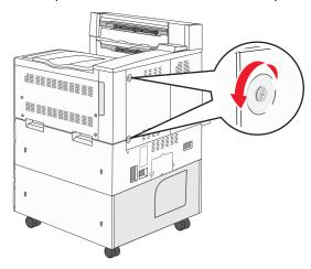
2 Remove the panel from the printer, and set it aside.
